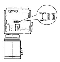
If the pan/tilt head is connected to the control panel with a cable longer than 300 meters, set the cable compensation switch on the pan/tilt head to the ON position in advance. If the distance between the pan/tilt head and the control panel is shorter than 300 meters, keep the switch in the original position (OFF). For details on shifting the switch, refer to the figure below or the Operating Instructions for Pan/tilt Head.
